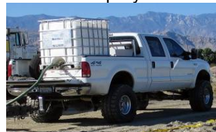
Pick-up Trucks with IBC Tote & Pumps
